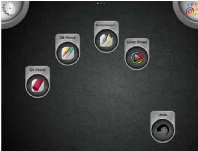
*The icons of the controls are conveniently positioned to match the shape of your hand so that each finger can quickly tap a control.*
