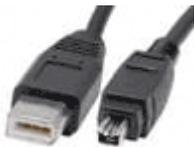
The special cable that connects your DV or D8 camcorder to your computer is called a Firewire cable. (It is also known as an iLink or IEEE 1394 cable.) This cable transmits digital data of both audio and video to your computer and can also send the same data back to your camcorder when you want to output your project back to tape. In addition to sending video data, it can also send commands from your computer to control the play functions of your camcorder.
