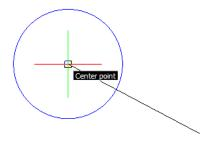
To help you identify valid esnap points, CorelCAD displays *tooltips* that identify geometric features, such as the "Center point" tooltip in the figure above. In all, CorelCAD has 13 entity snaps; the tutorials in later chapters make use of many of them.
